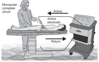
Fig. 1: Pathway of monopolar current
