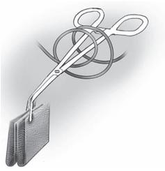
Fig. 13: Capacitance due to wrapping of monopolar code around artery forceps
