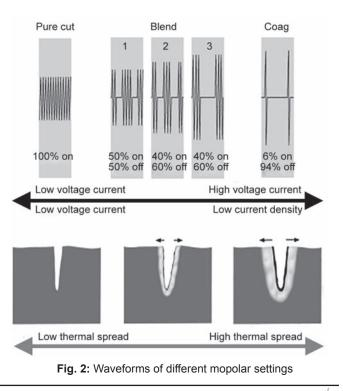
waveform is used in either contact or noncontact mode, yielding desiccation or vaporization respectively. Cut waveform is a continuous sinusoidal waveform with current flowing 100% of the time (duty cycle), coagulation waveform is an intermittent or "damped" waveform where the duty cycle is reduced, and blend waveforms are also intermittent waveforms, but with interrupted duty cycle.
