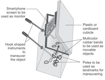
Fig. 1: Schematic diagram of the apparatus
