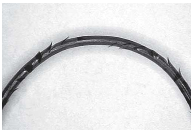
Fig. 1: Bidirectional barbed suture with barbs that change direction in the middle 17
