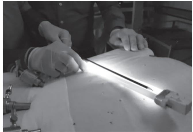
Fig. 12: Glowing of bulb due to capacitive coupling from monopolar hook
